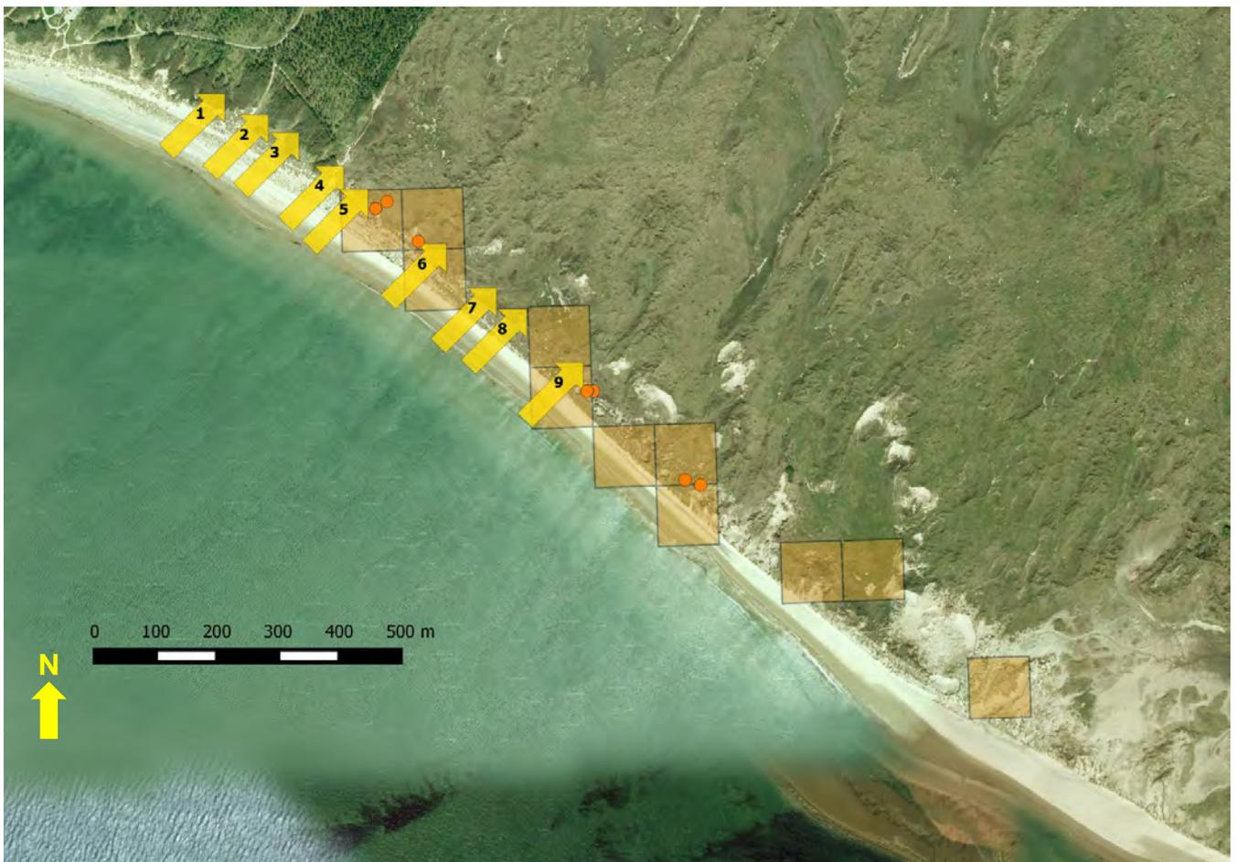
**Map 8:** Location of re-mobilisation notch works in relation to sand lizard records. Yellow arrows = location of notches. Orange dots = September 2015 sand lizard records. Orange squares = 2010-2014 sand lizard records.
