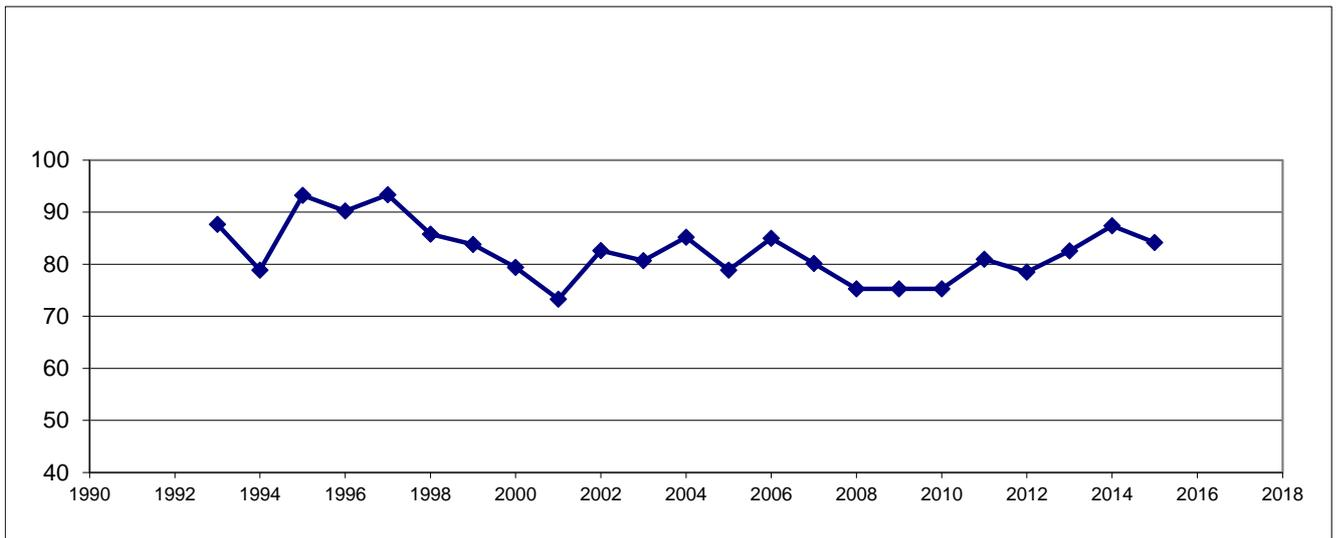
The maximum gust recorded for 2008, 2009 & 2010 was exactly the same (75.28 knots). It is possible the bearings were faulty. The bearings were replaced in 2011 and higher gusts are now being recorded. 2015 saw a maximum gust of 84.17 knots.
