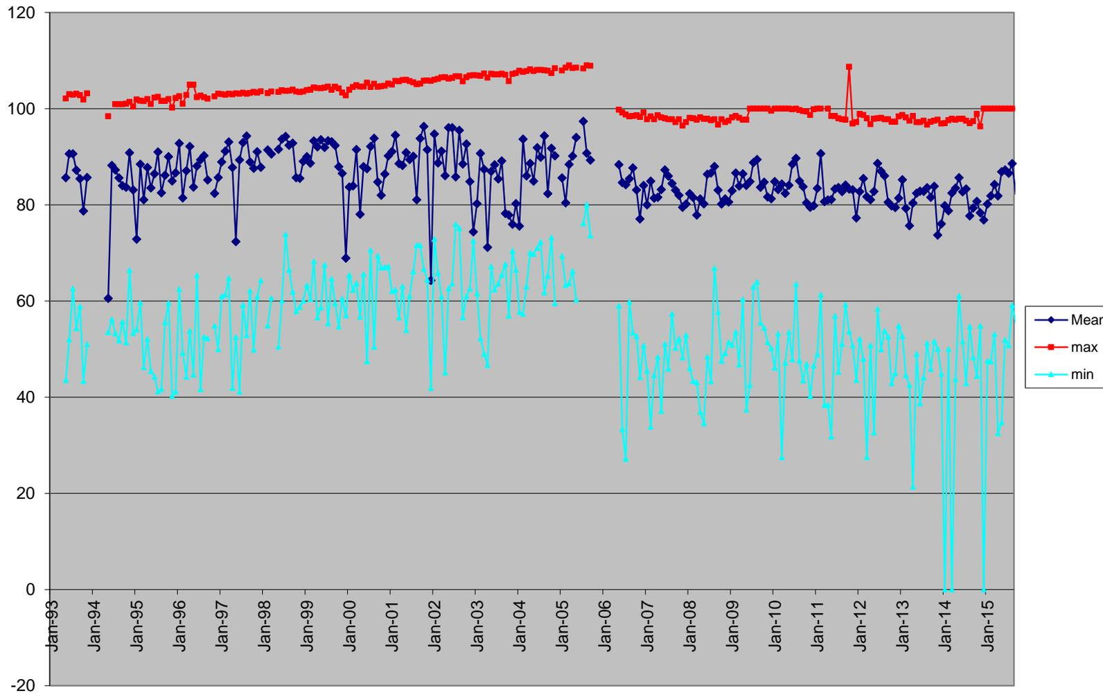
The increasing trend in relative Humidity from 1997 – 2005 may well be due to equipment error. From 2006 onwards there is no obvious trend.
