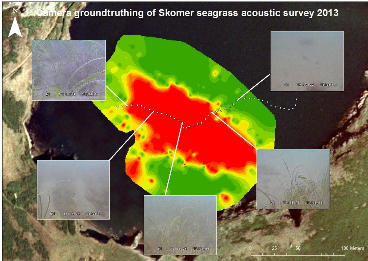
Images obtained during camera drift (dotted line) over eelgrass bed – the acoustic signal for seagrass was verified by the images from a towed camera.
