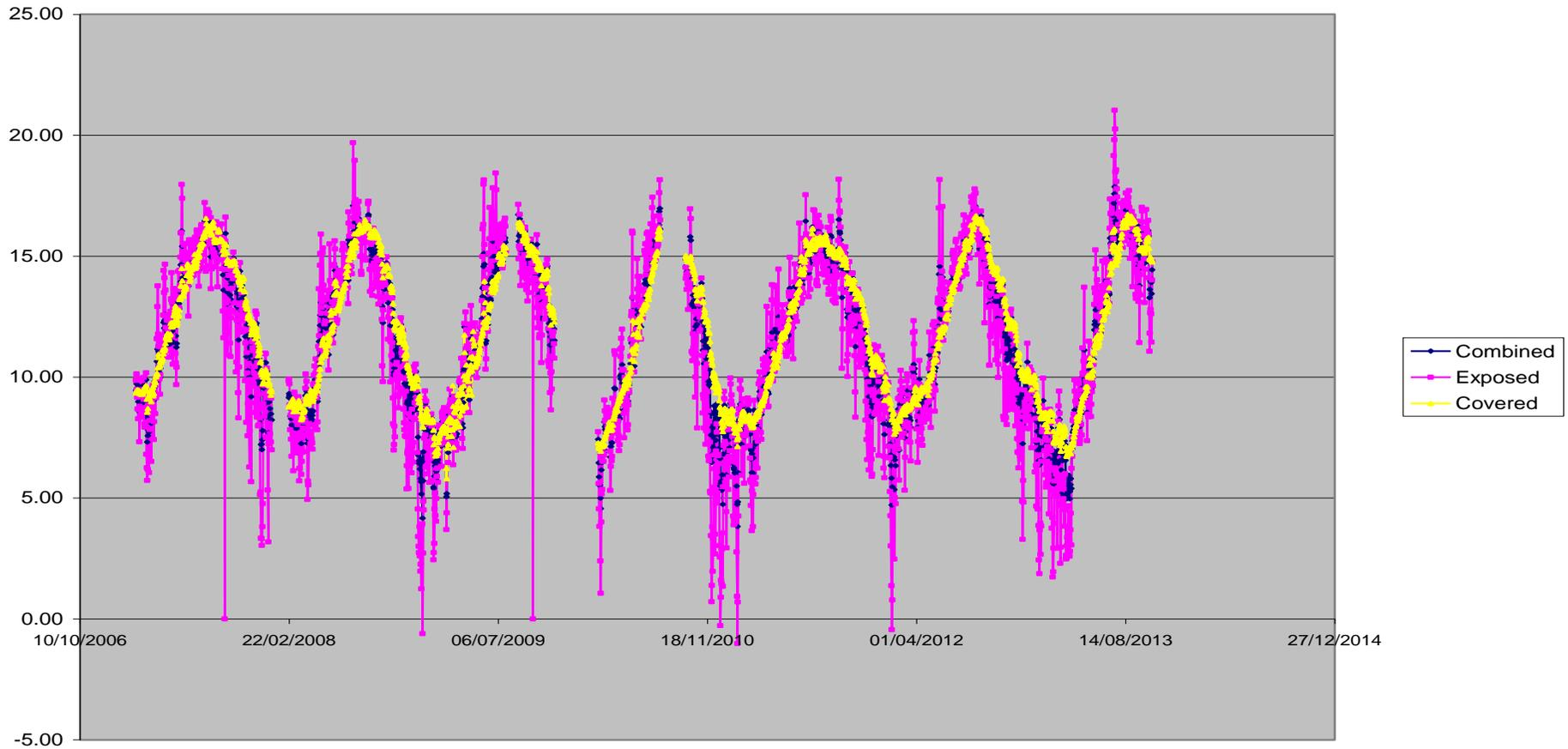
The pink data represents the air temperature (logger out of the water). The yellow data is sea temperature (logger covered by the tide).
