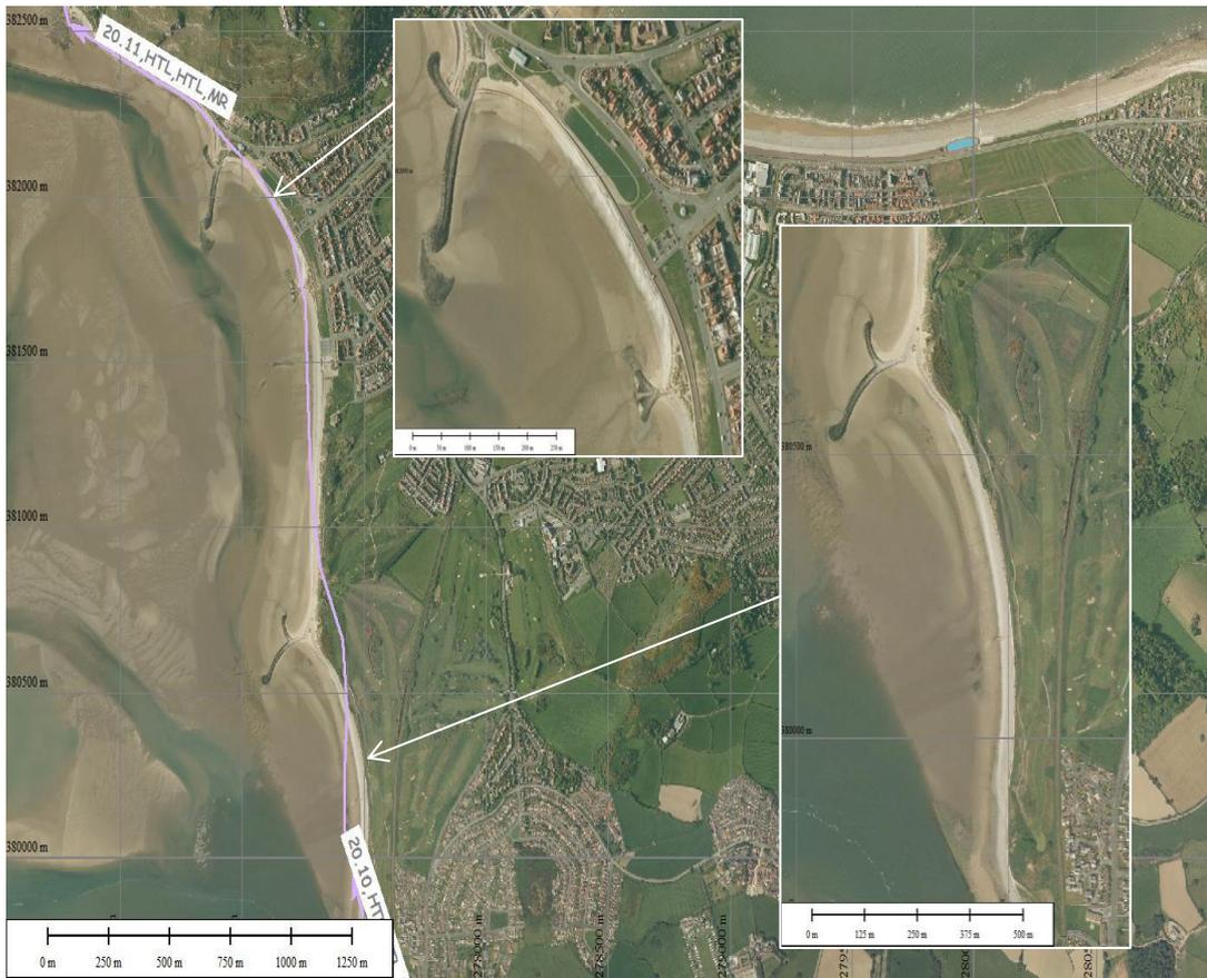
Figure 19. Deganwy North and Llandudno West Shore, showing areas of dune formation around the stem of two fishtail groynes built during the early 1990s
